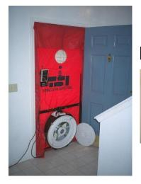
A blower door is used to identify air leaks in the home and ductwork system, then our expert weatherizes the home to decrease drafts and improve your heating and cooling costs!
