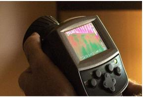
Our certified thermographer can use an infrared camera to scan the walls, ceiling, and floor joists of your home to identify areas of missing insulation. This technology can also identify air moving within wall cavities, allowing us to find problems that the blower door can not identify.
