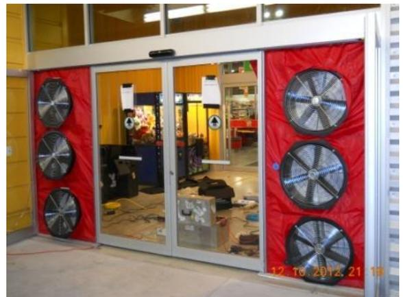
TSI can measure the total air leakage rate of a large building AND identify individual air leakage sites.
