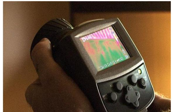
Our certified thermographer can use an infrared camera to scan the walls, ceiling, and floor joists of your home to identify areas of missing insulation. This technology can also identify air moving within wall cavities, allowing us to find problems that the blower door can not identify.
