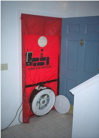
A blower door is used to identify air leaks in the home and ductwork system, then our expert weatherizes the home to decrease drafts and improve your heating and cooling costs!
